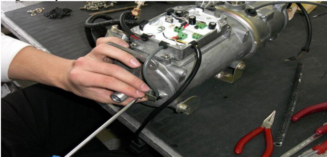
Fig. 7 - Overheating sensor installation and dismantling
