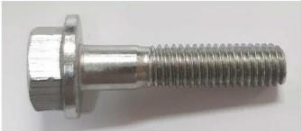
Bolt DIN 6921-10.9 Hex flange bolt. Length 35 Bolt securing intermediate shaft to camshaft
