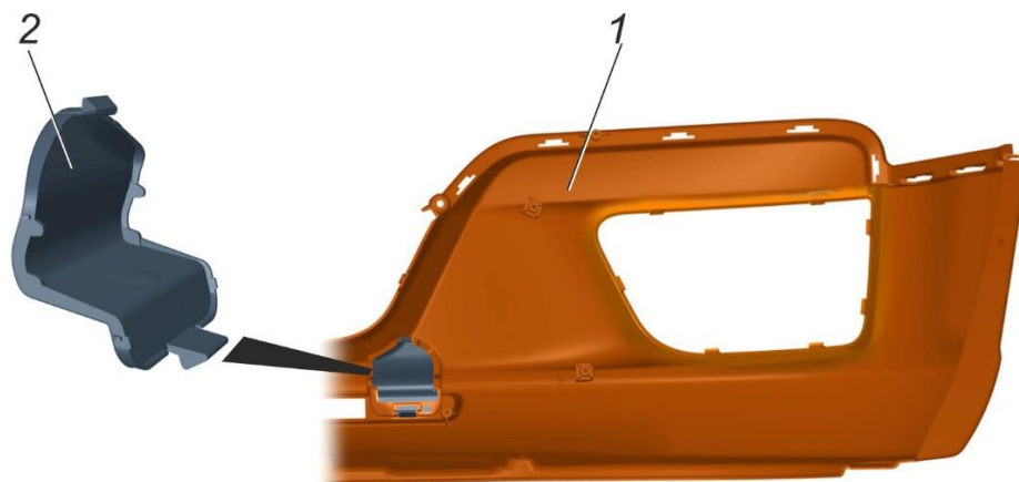
Fig. 8.16. Fasteners securing hatch covers to front bumper lower panel: 1 – front bumper lower panel; 2 – hatch cover
