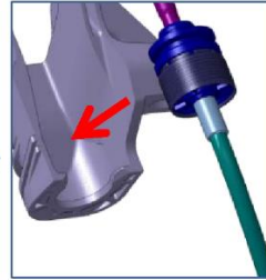
Insert the bushing into the master support body with the slid off cover.
