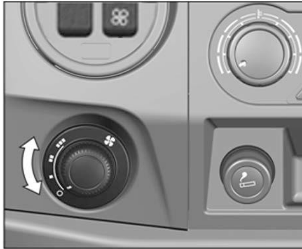
Fig. 7.36. Auxiliary heater switch installation
