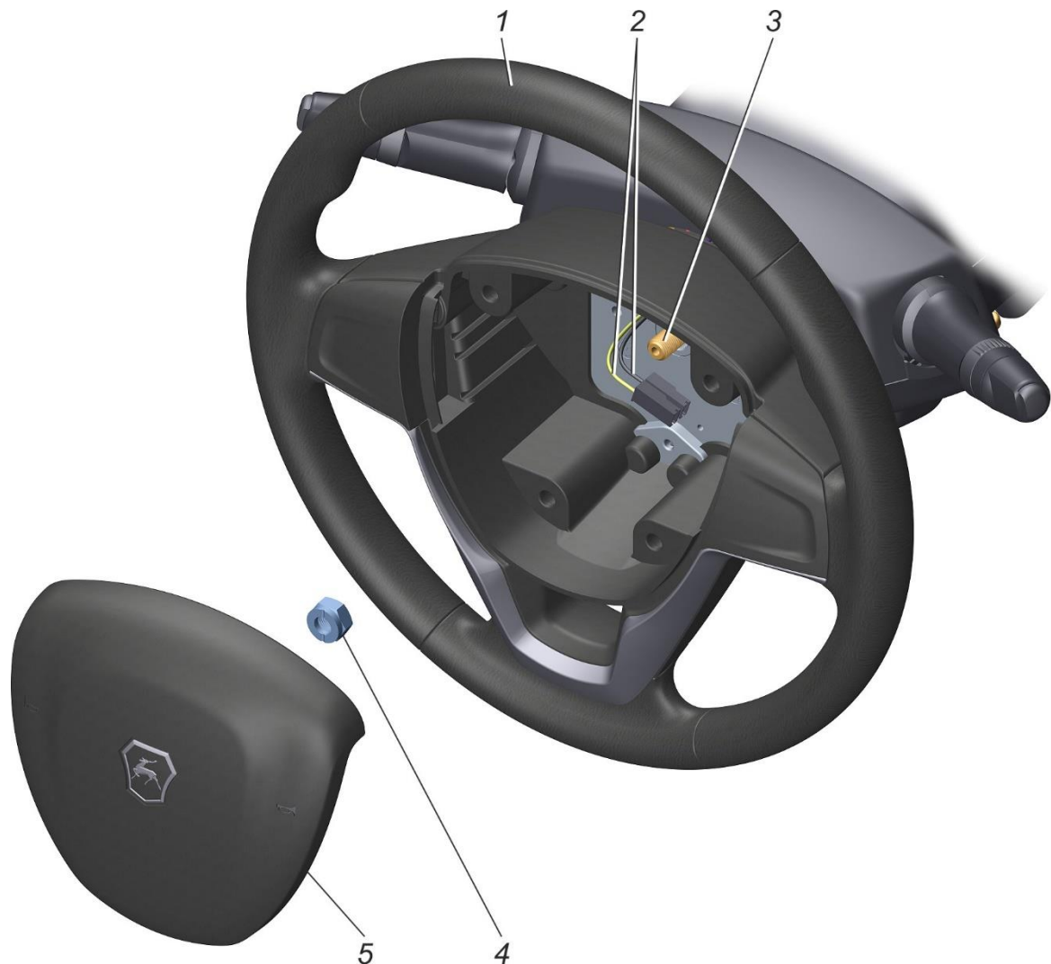
Fig. 5.12. Steering wheel: 1 – steering wheel; 2 – current transfer device wires to horn switch; 3 – steering column shaft; 4 – nut; 5 – decorative molding
