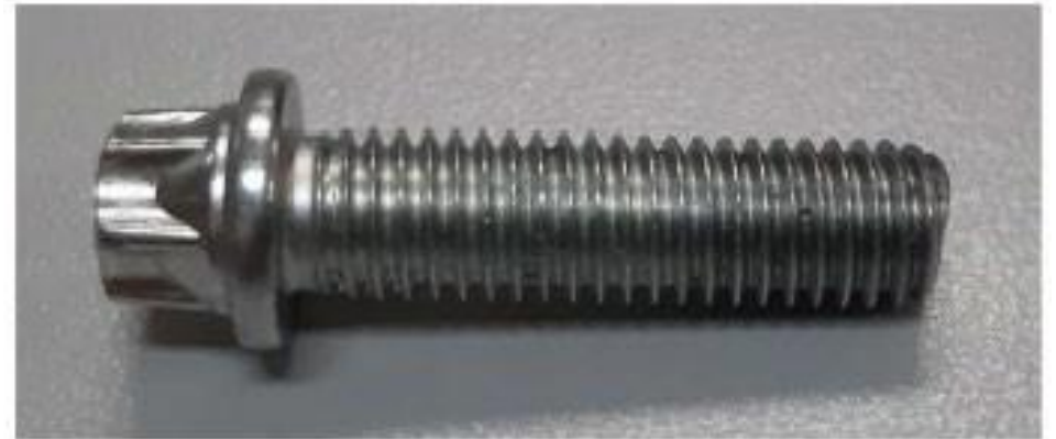
Bolt DIN 34800 M8x30 10.9 Bolt securing intermediate shaft to steering column
