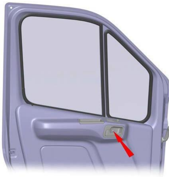
Fig. 8.23. Lock internal drive socket screw
