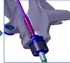
Insert the bushing into the master support body with the slid off cover.
