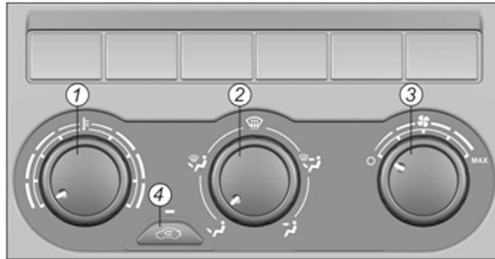
Fig. 8.45. Heating and ventilation control board: 1 – air temperature regulator knob; 2 – air flow distribution regulator knob; 3 – heater fan speed control knob; 4 – air recirculation mode on/off button
